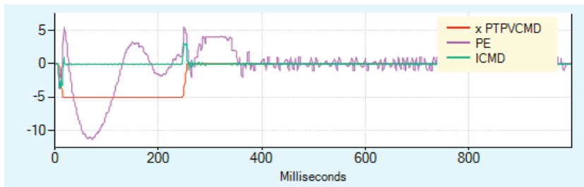
Figure 8-21. ICMD and PE Poor Result
